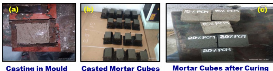
Fig. 3. (a-c) Casting of mortar cubes in moulds and prepared samples.
