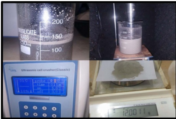
Fig. 2. Preparation of Ceno-PCM.
