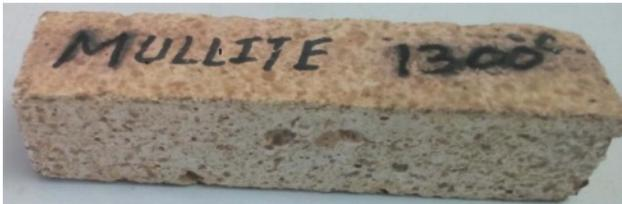
**Fig. 3.** Gel bonded castable brick.
