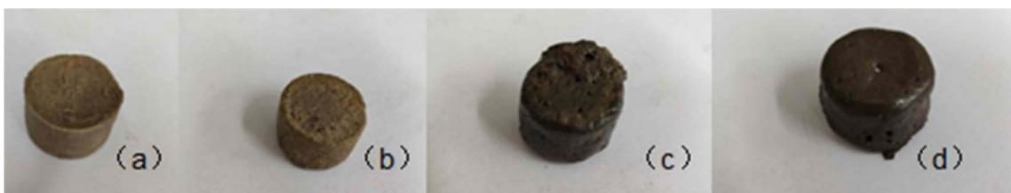
**Fig. 3.** Surface morphology of 10% Na<sub>2</sub>CO<sub>3</sub> at different temperatures: (a) 900 °C, (b) 950 °C, (c) 1070 °C and (d) 1090 °C.
