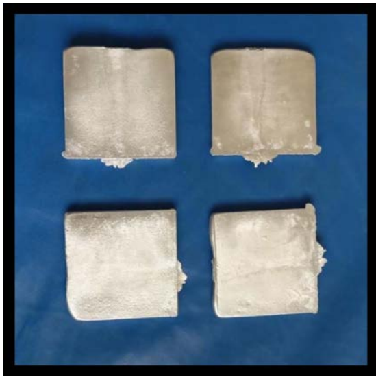
Fig. 1. AA6063 with 5 wt% SiC and 5 wt% B 4 C hybrid composites.
