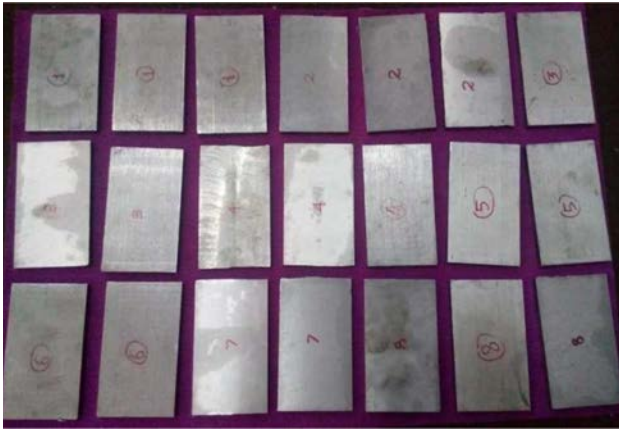
Fig. 4. Prepared AMMHC plates for FSW process.
