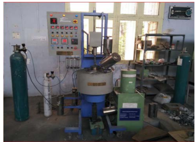
Fig. 4. Stir casting setup.
