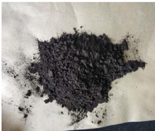
Fig. 1. Manganese tailings sample powder.
