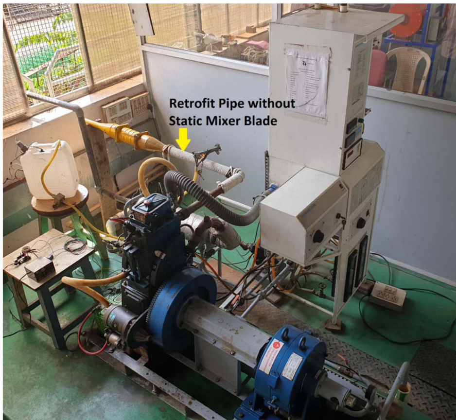
Fig. 4. Picture of engine test bench setup with retrofit system
