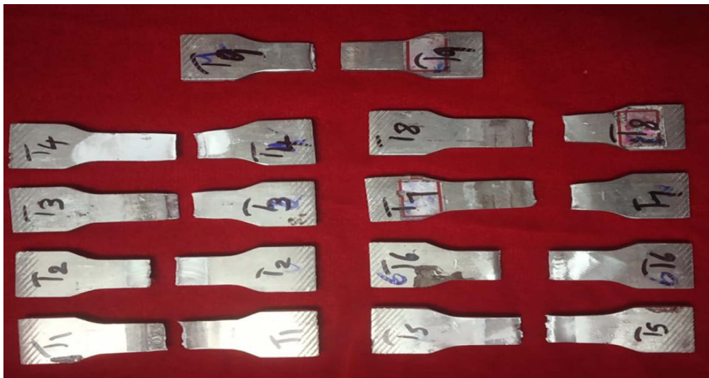
Fig. 3. Fractured tensile specimen of FSWed AA5052.
