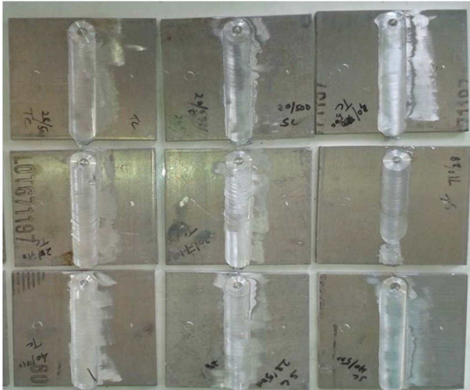
Fig. 2. Friction stir welded joints of AA5052.
