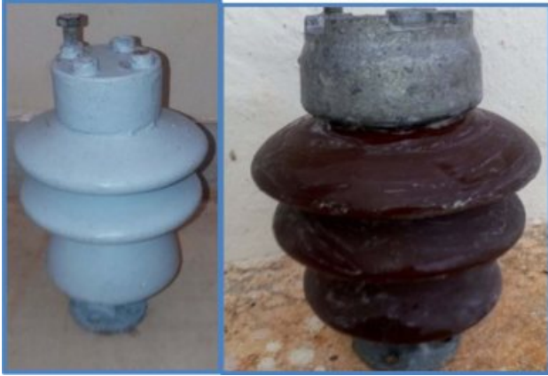
Fig. 4. RTV Silicone and Epoxy Resin Coating.
