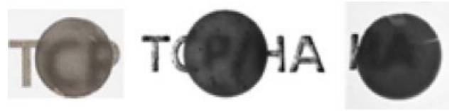
Fig. 4. A translucency example for the sintered specimens at 1,100 °C for 2 h using the prepared calcium phosphates powders from the different precursor Ca/P ratios (TCP (Ca/P = 1.30), TCP/HA (Ca/P = 1.50), and HA (Ca/P = 1.67)).
