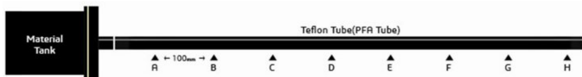
Fig. 1. Analytical equipment for determining material extrusion properties using DIW 3D printer material feed system.
