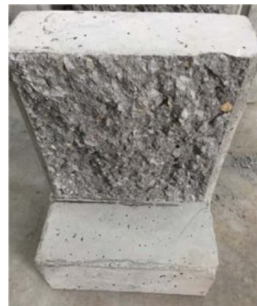
Fig. 14. Failure surface of the shear specimen.
