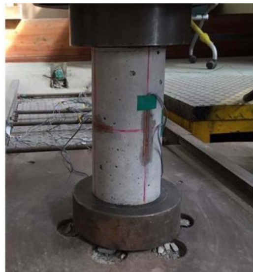
Fig. 9. Concrete compressive strength test.
