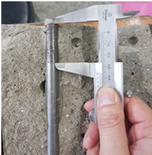
Fig. 2. Measurement of corrosion-ratio after splitting of specimens.
