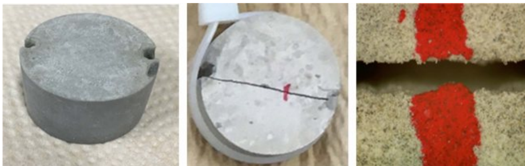
Fig. 3. Assessing self-healing through cracks in cementitious paste.
