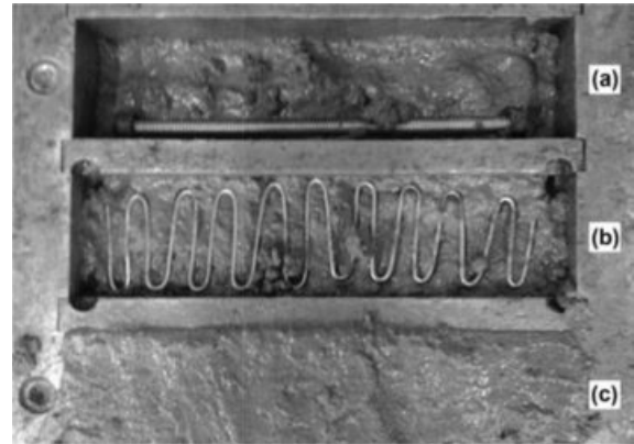
Fig. 8. Reinforcement used in mortar specimens (a) flexural reinforcement, (b) shear reinforcement and (c) surface finish [7].
